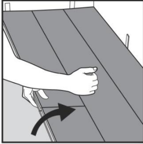
Fig 11. Separate the whole row by carefully lifting up and release the whole row. Fold up the row and release the whole long side.
